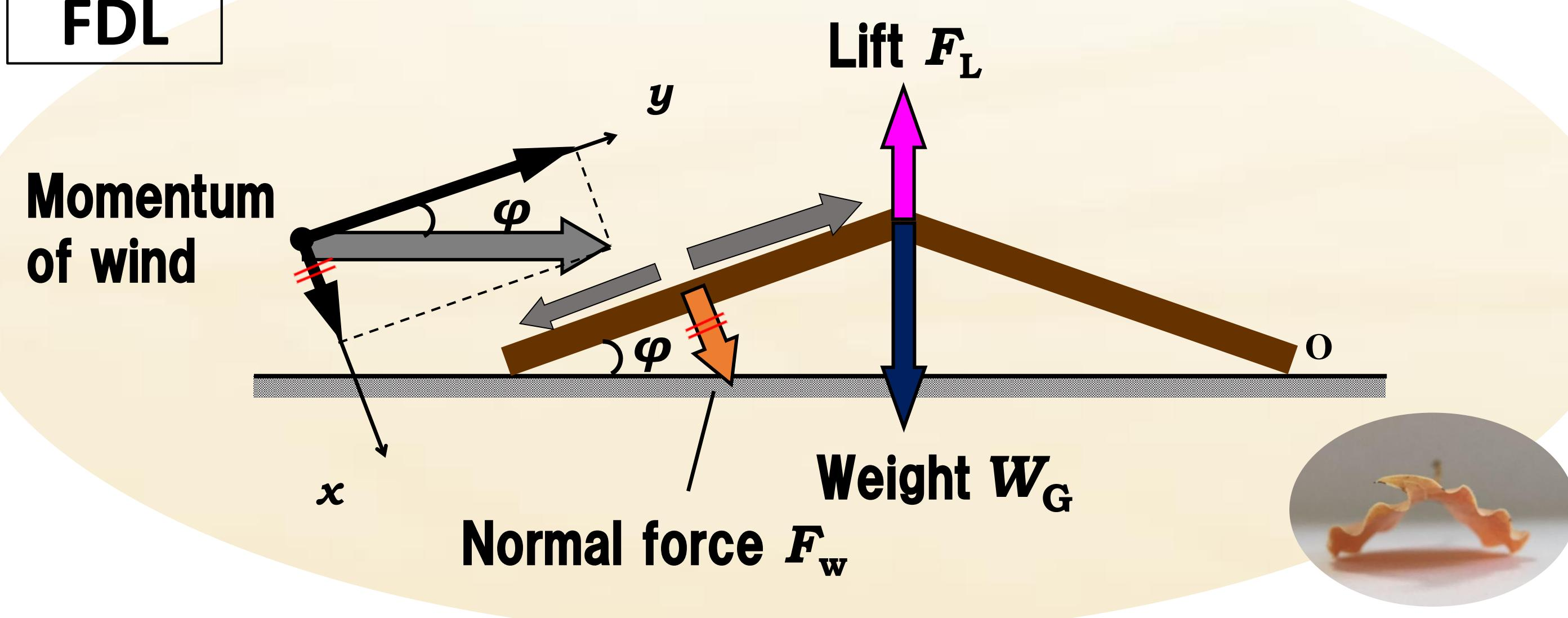
Fig.7 Normal force and lift generated by wind
