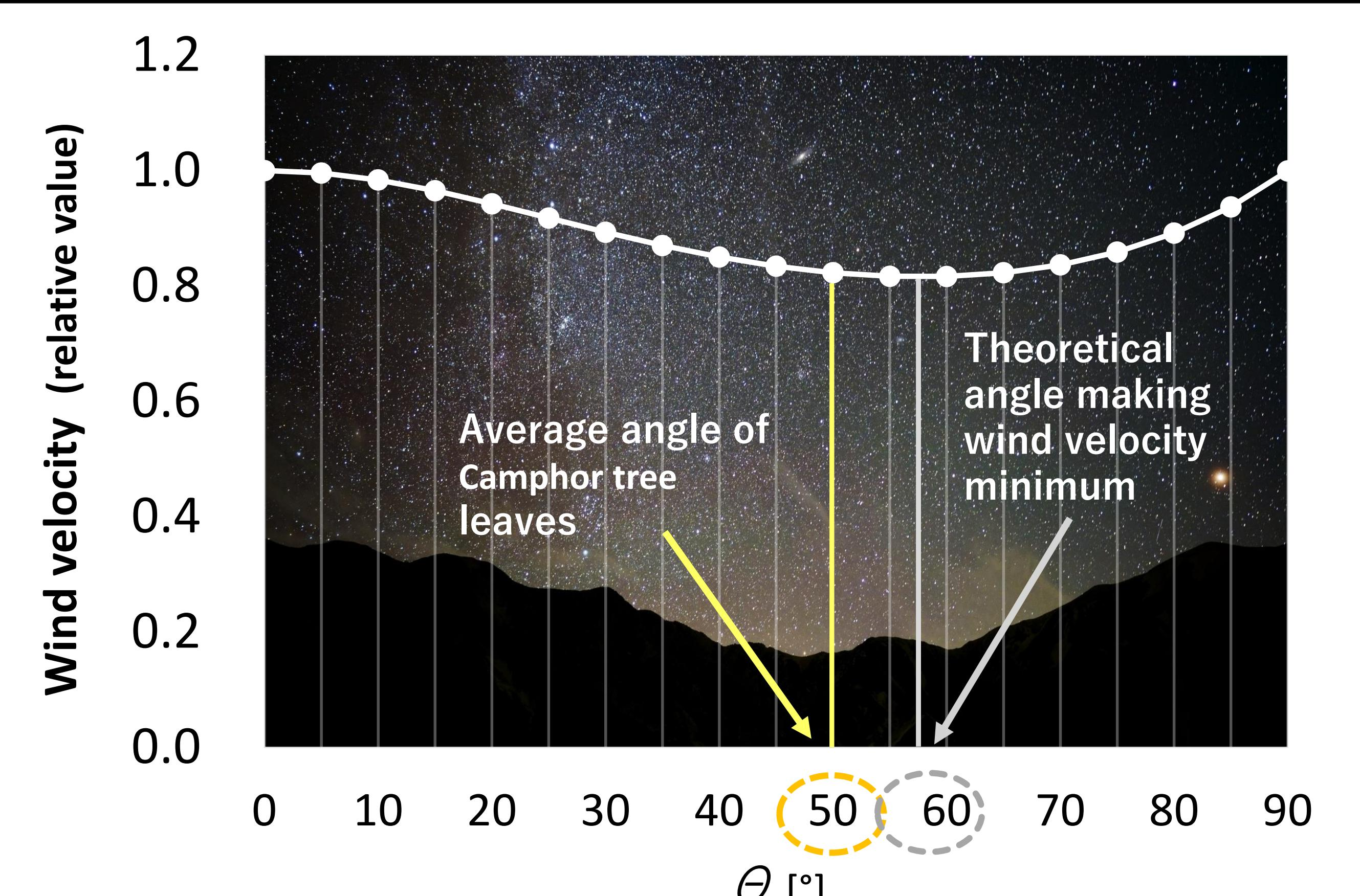
Fig.9 Relation between curvature angle of FUL and wind velocity for flipping
